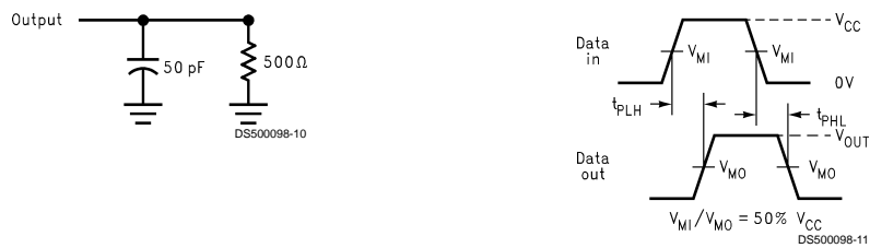
FIGURE 3. t_{PHL} , t_{PLH} Test Load and Waveforms B_1 – B_8 to A_1 – A_8 , C_{14} – C_{17} to A_{14} – A_{17} , HLH_{IN} to HLH
