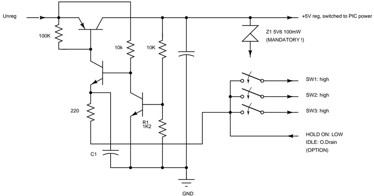
NOTES: 1. R1 adjusts output voltage. 2. C1 adjusts turnoff time (delayed turnoff). 3. Z1 is MANDATORY and its voltage should be HIGHER than the regulated output voltage of the circuit.
