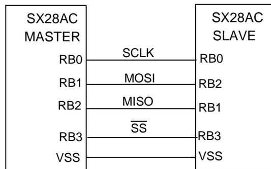
Figure 6-1. SPI Master-Slave Demo Program Configuration
