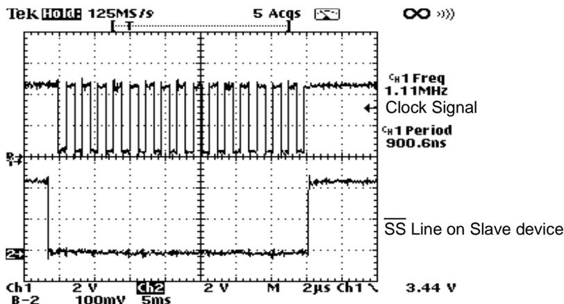
Figure 6-2. Clock and  $\overline{SS}$  line on slave device
