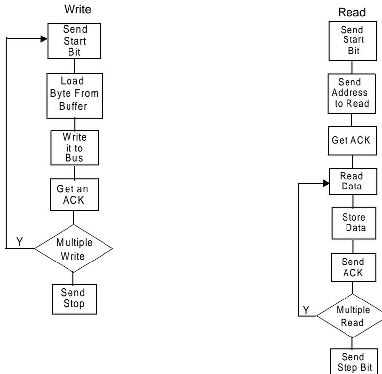
Figure 4-2. I<sup>2</sup>C Master State Machine (Multiple read/write is default “N” in demo code)
