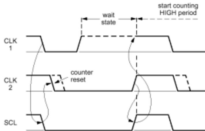
Figure 3-4. Clock Synchronization During the Arbitration Procedure
