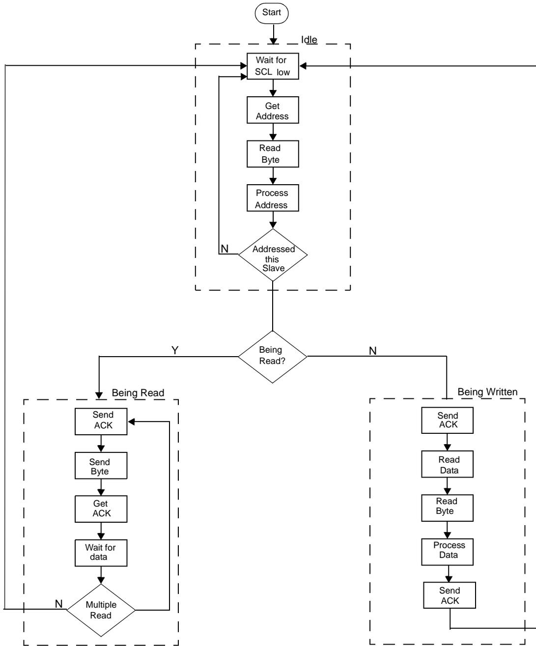
Figure 4-1. I<sup>2</sup>C Slave State Machine
