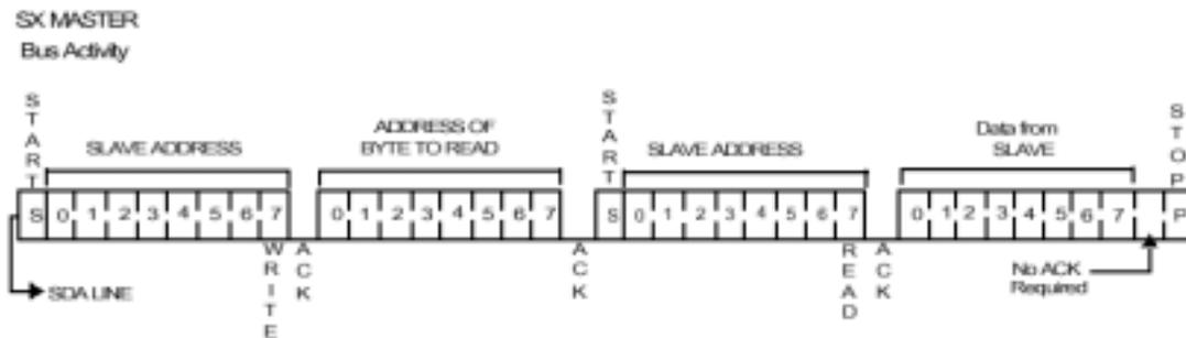
**Figure 6-2. I<sup>2</sup>C Master Reading Data from Slave**
