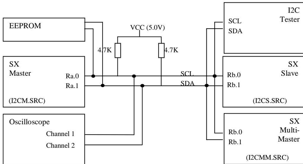
**Figure 7-1. Overview of the Test Environment**
