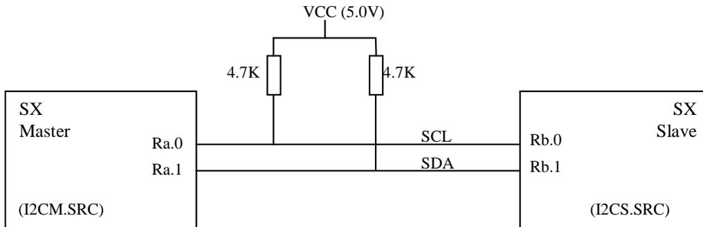
**Figure 6-1. I<sup>2</sup>C Virtual Peripheral Demo Connection Diagram**
