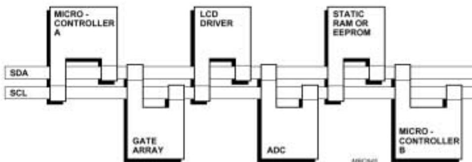
Figure 2-1. I<sup>2</sup>C-Bus Using Two Microcontrollers
