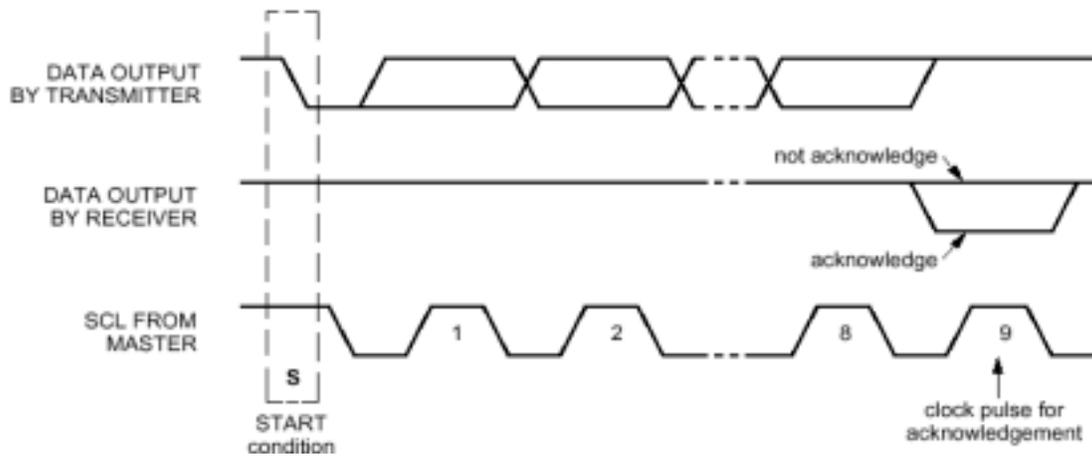
**Figure 3-3. Acknowledge on the I<sup>2</sup>C-bus**
