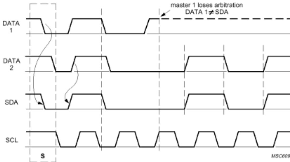
Figure 3-5. I<sup>2</sup>C Arbitration Procedure of Two Masters
