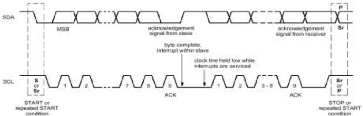
Figure 3-2. Data Transfer on the I<sup>2</sup>C-bus
